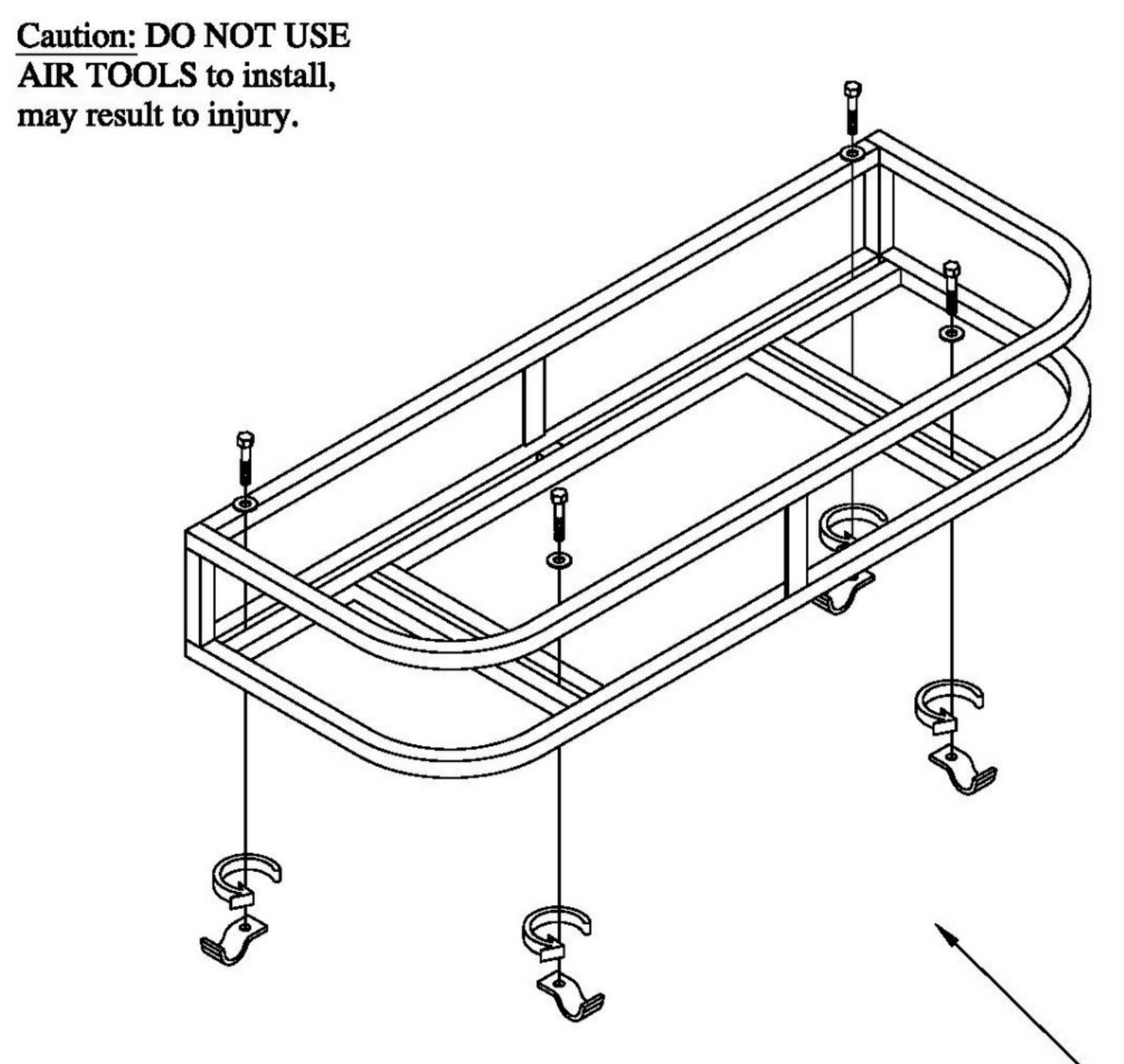
THE CLIPS WILL MOUNT EITHER WAY DEPENDING ON THE ORIGINAL RACK DESIGN.
